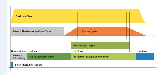
Graph displaying the measurement with system triggering of the flash (example) Method (b)
