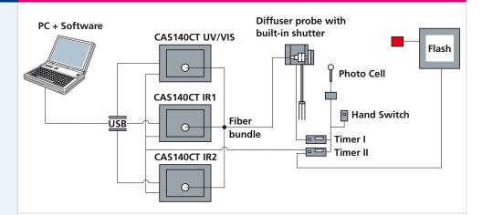
Multiple CAS140CT array spectroradiometers simultaneously measure the complete spectral irradiance of a flash. The diffuser probe is equipped with a fast mechanical shutter to define the measurement window.
