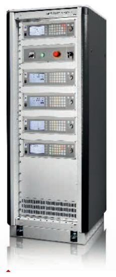
Optional 19" switch cabinet with space for further source meters and measuring instruments.
