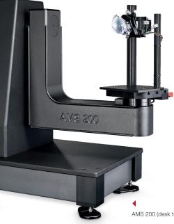
The AMS 200 of the Optronik line is a Type A goniophotometer conforming to CIE 121-1996 and IES LM-75-01. It is suitable for measuring the photometric and colorimetric data of small to mediumsized lamps and modules with directed radiation distribution, e.g. signal lamps, vehicle, bicycle and motorcycle headlamps or headlamp modules and reflectors of all kinds.
