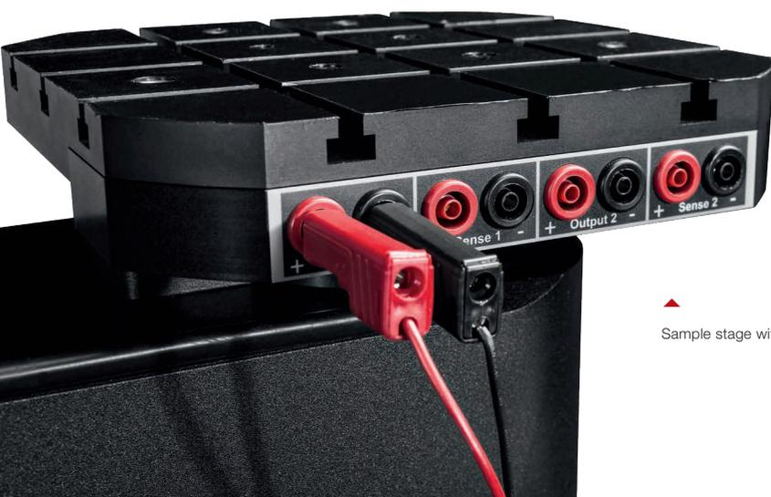
▲ Sample stage with electrical connections.
