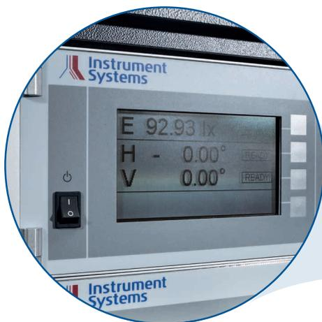
▲ AMS controller display showing angle position and active measuring channel with unit.
