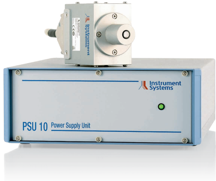
► ACS-570 series of LED calibration standards. The compact power supply and TEC-control unit PSU 10 ensures a fast temperature regulation, as well as a high stability of the supply current.
