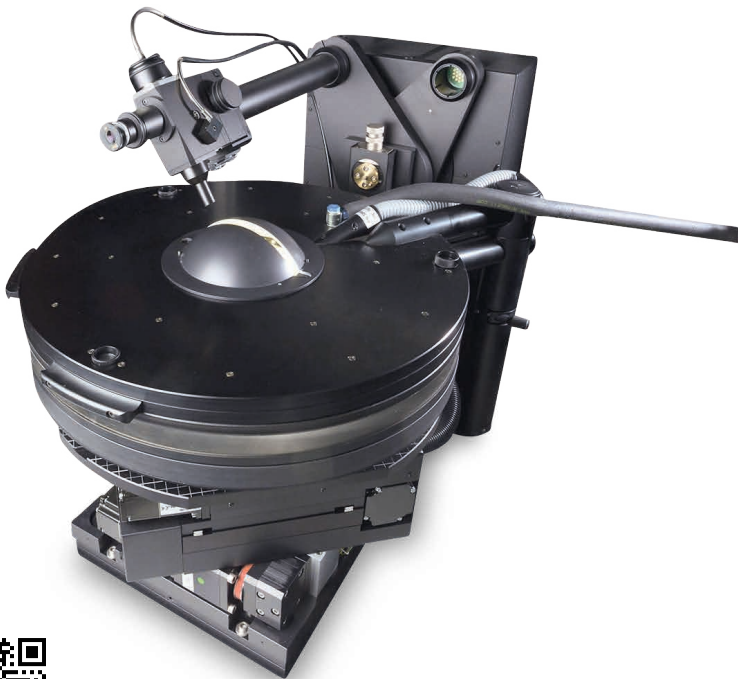
Fig. 7: The heat-cool system HCS-3B exposes the DUT to temperatures from -40\text{ }^{\circ}\text{C} to 105\text{ }^{\circ}\text{C} .
