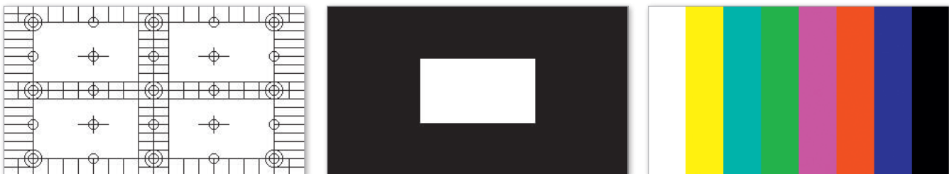
Fig. 12: Generation of test and alignment patterns by connecting pattern and video generators through the native device control interface (DCI advanced)
