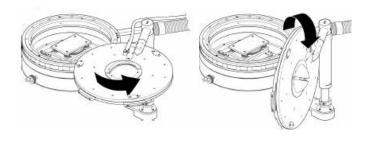
Convenient open and close mechanism of the HCS-3B.
