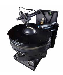
The HCS-3B is an optional mechanical component for the DMS 803, DMS 505 and DMS 201 display measurement systems. This heat-cool system – available in different variants – enables temperature-dependent measurements of optical display properties and conformance testing. It is used to measure electro-optical and switching characteristics under arbitrary directions of observation as well as angular scans over the viewing cone.
