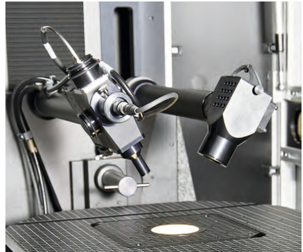
Figure 13: VADIS mounted at the reflective illumination arm of a DMS 803.
