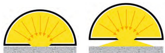
Figure 6: Illuminance of DUT in close proximity to the bottom plane of the DHS (left). Illuminance of DUT removed from the bottom plane of the DHS (right).
