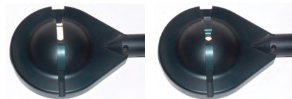
Figure 3: Gloss-trap slit partially closed (SCI/SPINC for microscope inclinations \geq 10^\circ ; left); gloss-trap slit closed (microscope inclination restricted to 0^\circ ; right).
