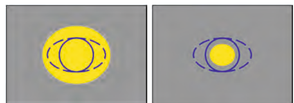
Figure 15: Measurement field (blue circle) overfilled: The illuminated area of the DUT (yellow) is larger than the measurement field (left). Measurement field (blue circle) underfilled: The illuminated area of the DUT (yellow) is smaller than the measurement field (right).
